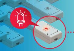
Senko's innovative Easy Trace Identification System offers a quick and accurate method of identifying the termination point of optical patch cords. Each end of a patch cord features an LC Connector with a flashing light source allowing technicians to visually trace individual patch cords from one end to the other without pulling or affecting the patch cord.
