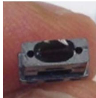
Figure B: Improper bead shown – Epoxy should not wick into the holes.
