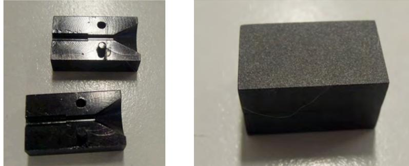
When assembled the fixture has two openings at either end. The small opening has a small straight internal diameter into which the pin tube is installed and held. The larger conical shaped opening at the opposite end is to guide fibers into the pin tube. See below.
