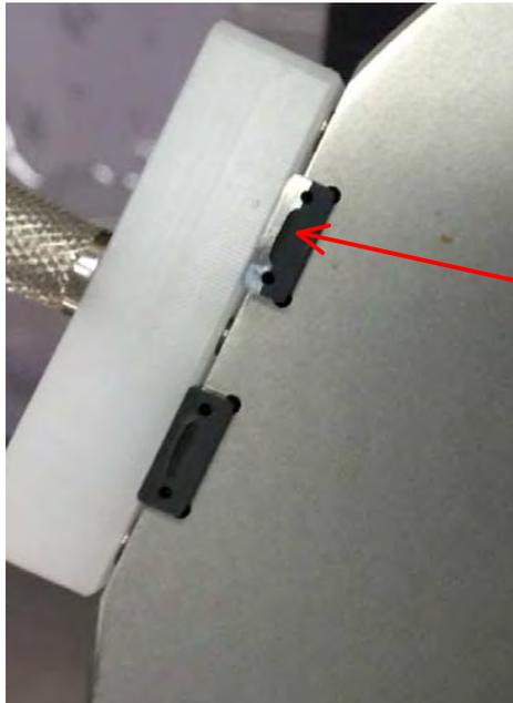
Here is can be clearly seen that the polished angle has reached the single row of fibers.
