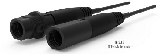
The IP-Solid SC Female Connector is a robust fiber optic connectivity solution designed for deployment in challenging environments that may include harsh temperatures, moisture, dust, and more. This hardened fiber optic connector is optimized for FTTH deployment. With its IP68 rated light-weight plastic body, the IP-Solid SC Connector can be terminated easily on various cable types including 4.8 mm round, flat drop, and the smaller footprint micro flat drop.
