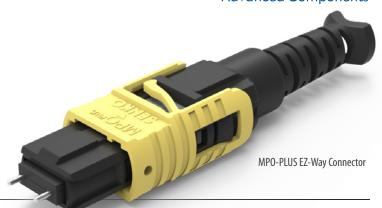
SENKO's soft-spring MPO-PLUS® EZ-Way™ connector is tailored for high-density scenarios where space is at a premium. Its compact design and push-pull boot are ideal for 800G dual belly-to-belly type transceivers and facilitate swift insertion and removal. The patented soft-spring housing design and reverse latch back post support enhanced mechanical strength while reducing the generation of plastic debris seen in traditional MPO, providing an improved user-friendly patching process.
