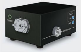
• Inspects 12 fiber in 2.6 seconds, 24 fiber in 4.5 seconds
