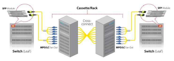
The SN® connector can simplify and reduce the overall cost of this structure, as SN® based transceivers are already broken out by having four (4) individual SN® connectors at the transceiver interface. To make a mesh fabric cross connection, it only requires SN® to SN® jumpers that can be connected point to point at the transceiver.
