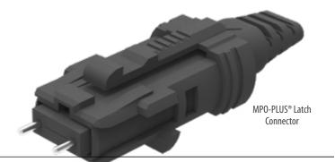
The MPO-PLUS<sup>®</sup> Latch connector features an innovative latch design for easier connection and disconnection than traditional push-pull MPO housings, while retaining the MPO-PLUS<sup>®</sup> oval spring and free-floating high-quality ferrules. It is compact, with a 20N spring for 24F ferrules, and includes a high-quality, low-loss ferrule. Note that a latch-compatible adapter is required.
