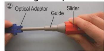
② Cleaning ends when the slider is pushed all the way. When pressure is relieved the slider naturally returns to its starting position, ready for the next cleaning. Pull out the cleaner from the adapter to end the cleaning process.
