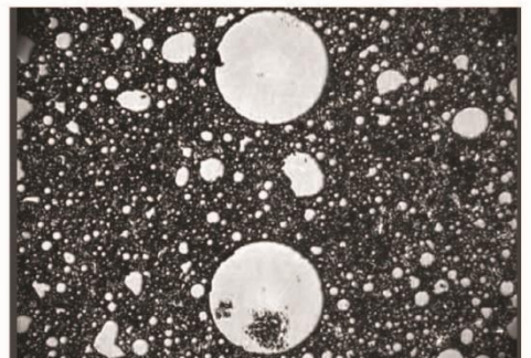
Segment of MT12 connector endface (SMX-Scopio)
