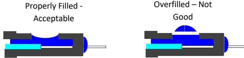
Figure 6: Proper epoxy amount on MT ferrule window (left) vs overfill (right)
