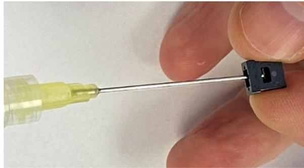
*Figure 4: Proper epoxy dispensing into MT ferrule*
