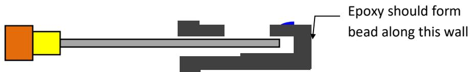
*Figure 3: Epoxy application using 20 AWG needle*
