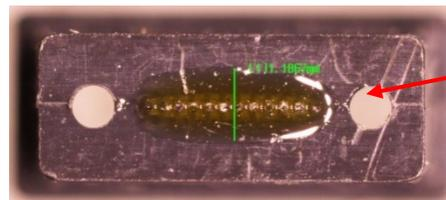
Ideal epoxy bead should be approximately 1.2mm or less in width
