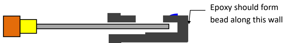
Figure 3: Epoxy application using 20 AWG needle
