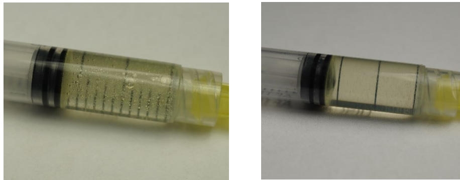
Figure 2: Epoxy on the left with air bubbles after mixing and on the right degassed in centrifuge
