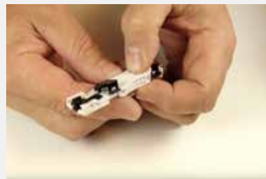
Push fiber into fiber holder
