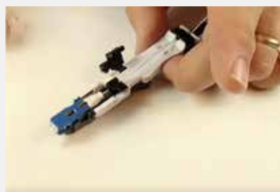
The connector is terminated
