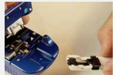
Set the cleaver for cutting
