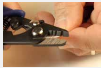
Strip fiber to correct length
