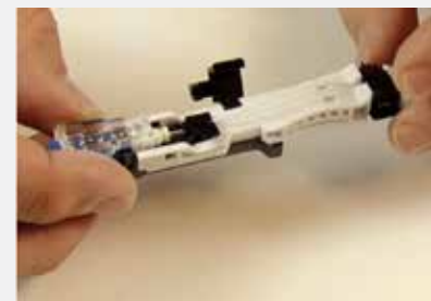
Remove wedge from connector
