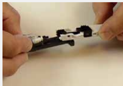
Insert assembly into connector holder
