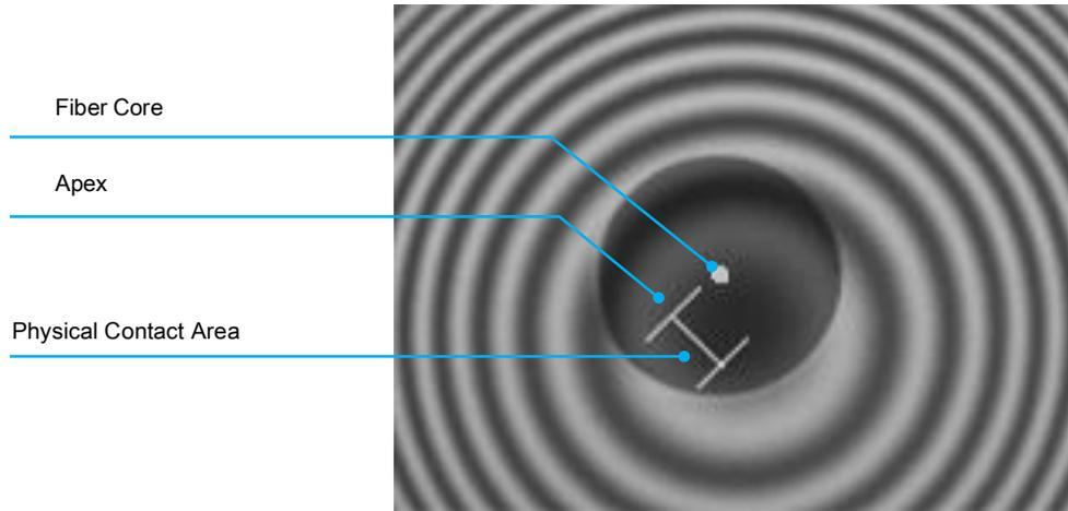
*Figure 6: Interferometry Image showing Apex Offset*
