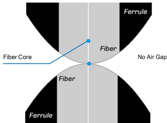
*Figure 7: Zero Apex Offset in perfect Physical Contact*
