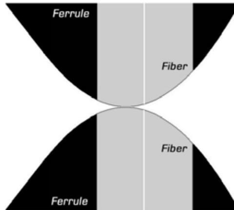
*Figure 8: High Apex Offset results in an Air Gap*
