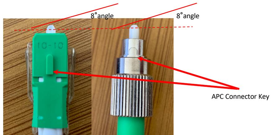
Figure 5: APC Angle with respect to Key
