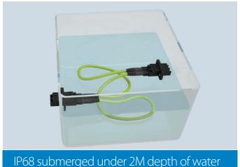
for 30 minutes and no water leakage
