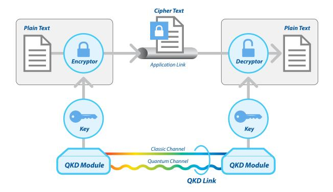
The basic elements of a QKD communication system are the transmitter and receiver (QKD modules), and a QKD link between them comprising a Classical Channel and a Quantum Channel. The Classical Channel is used for data exchange between the QKD modules, while the Quantum Channel transmits quantum signals such as single or entangled photons, from which the cryptographic keys are derived.
