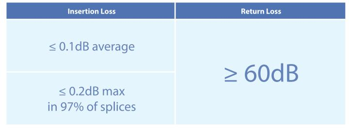
Insertion & Return Loss of Fusion Splices as per IEC Standards IEC 61300-3-6 and IEC 61300-3-7
