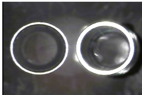
Figure 5: Example of thin wall (poor quality) left vs. thick wall (good quality) right
