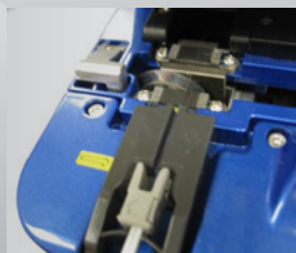
▶ 3 Cleaving of the fiber
