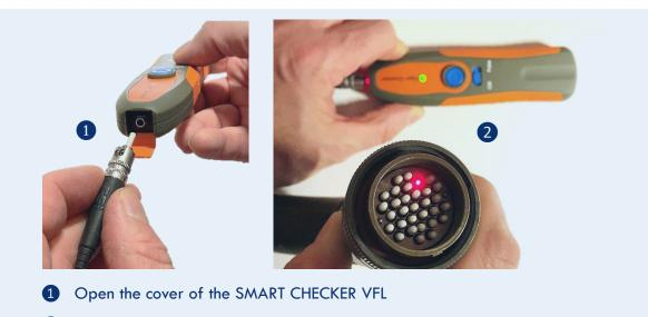
2 Insert MIL ST into the SMART CHECKER VFL and push the blue button
