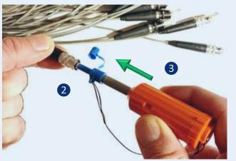
3 Push the cleaner 1X until it bottoms out for cleaning the endface
