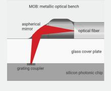
Metallic PIC Connector in electro-optical transceiver
