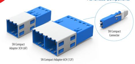
SN° compact adapters are available either as a 3-channel (6 fibers) or 6-channel variant (12 fibers). The 3-channel type is designed to fit to legacy hardware incorporating the SC simplex (LC duplex) cut-out, and the 6-channel version is designed to fit legacy hardware incorporating the SC duplex (LC quad) cut-out.
