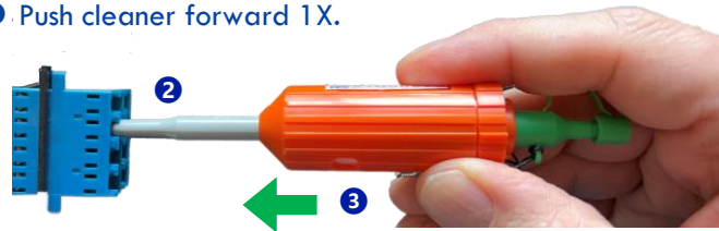
Cleaning In adapter LC end faces.
