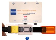
Remove the prospective end cap from the MPO assembly and clean the connector.
