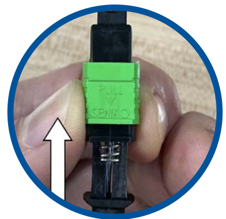
Figure 8 Proper usage of MT male dummy ferrule to aid MPO housing installation.
