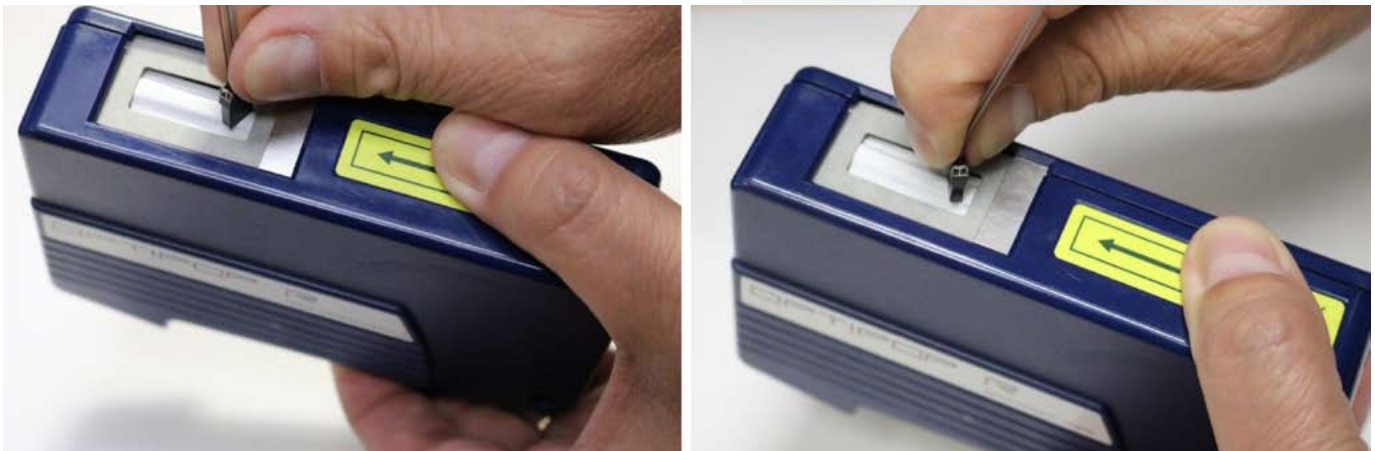
Figure 9 Male MPO proper cleaning using Optipop cassette.
