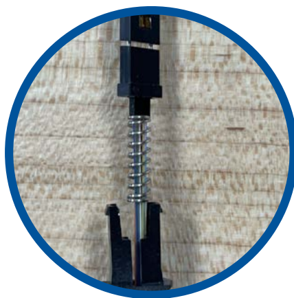
Figure 8 Proper usage of MT male dummy ferrule to aid MPO housing installation.
