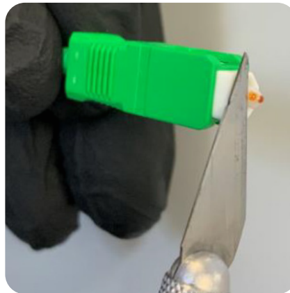
Figure 4 Excess epoxy from the sides can be removed by blade.
