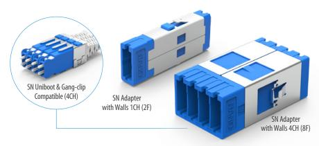
SENKO's SN° adapters with walls are available either as a 1-channel (2 fibers) or 4-channel variant (8 fibers). The single channel is designed for applications requiring the separation of individual optical channels such as coherent optics or wave-splitting. The 4-channel version is designed to maximize port density within patch panels.
