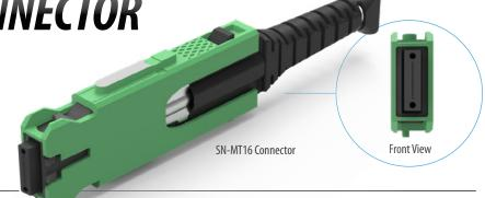
SENKO's SN°-MT16 is an extension of the SN° range and incorporates a single, compact SN-MT ferrule with 16 x 200 µm fibers in a single row. Subsequently, the SN°-MT ferrule can achieve 2.7 times the density of MPO16 whilst leveraging the same proven alignment methods. This combination ensures low-loss performance for singlemode and multimode APC applications whilst delivering optimized patch-panel density required in today's Hyperscale data centers.
